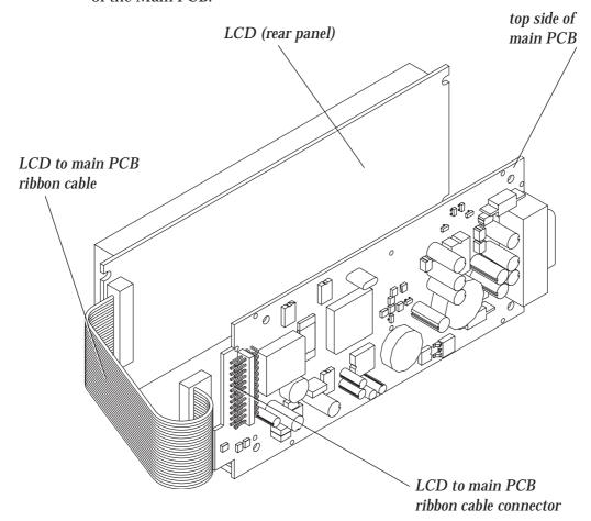
Figure 4.9 Connecting the LCD to Main PCB Ribbon Cable
