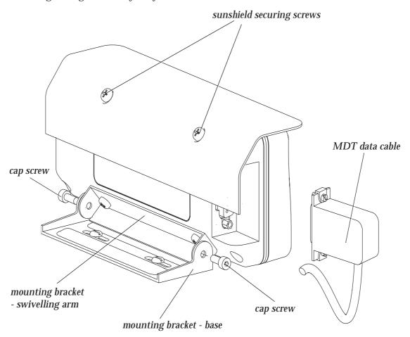
Figure 4.2 Removing the MDT from its Working Installation
