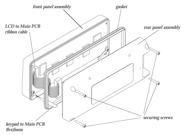
Figure 4.3 Disassembling the MDT - Rear View
