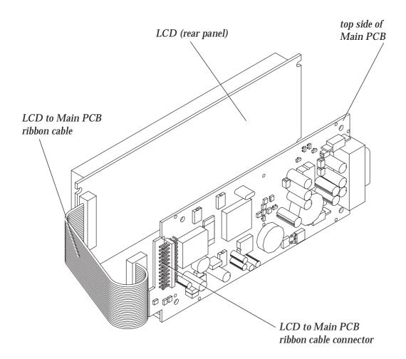
Figure 4.5 Disconnecting the LCD to Main PCB Ribbon Cable
