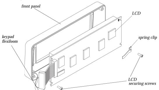
Figure 4.6 Separating the LCD from the Front Panel - Internal View of Front Assembly
