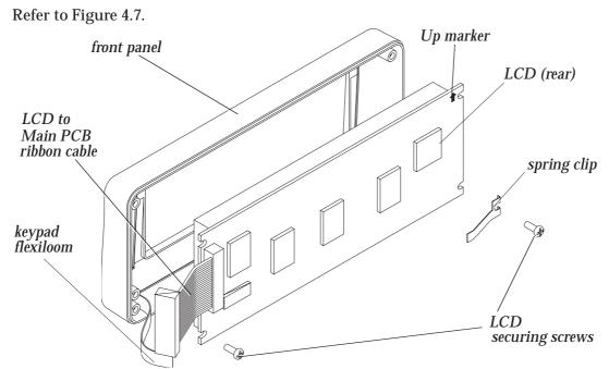
Figure 4.7 Fitting the LCD to the Front Panel - Internal View of Front Assembly
