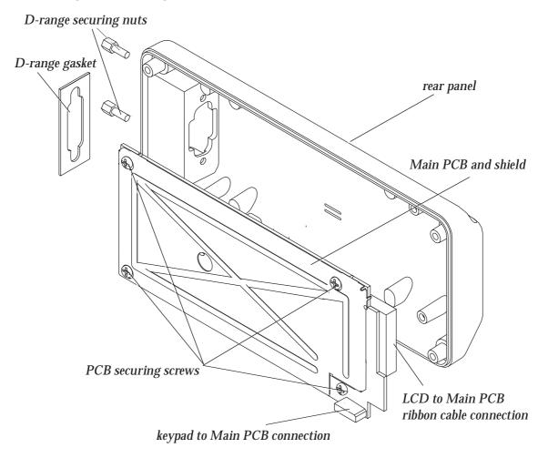
Figure 4.4 Separating the Main PCB from the Rear Panel - Internal View
