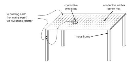
Figure 4.1 Typical Antistatic Bench Setup
