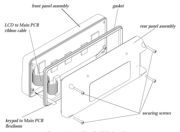
Figure 4.10 Assembling the MDT - Rear View
